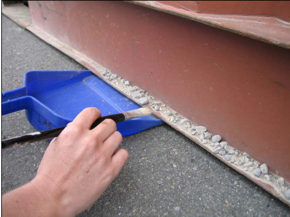
Figure 4.10 Dirt, stones and other contaminants found on the base plates of containers. This shipping container (1809097) had been in South Canterbury as part of a drilling project (Photograph by A. Fortune).
