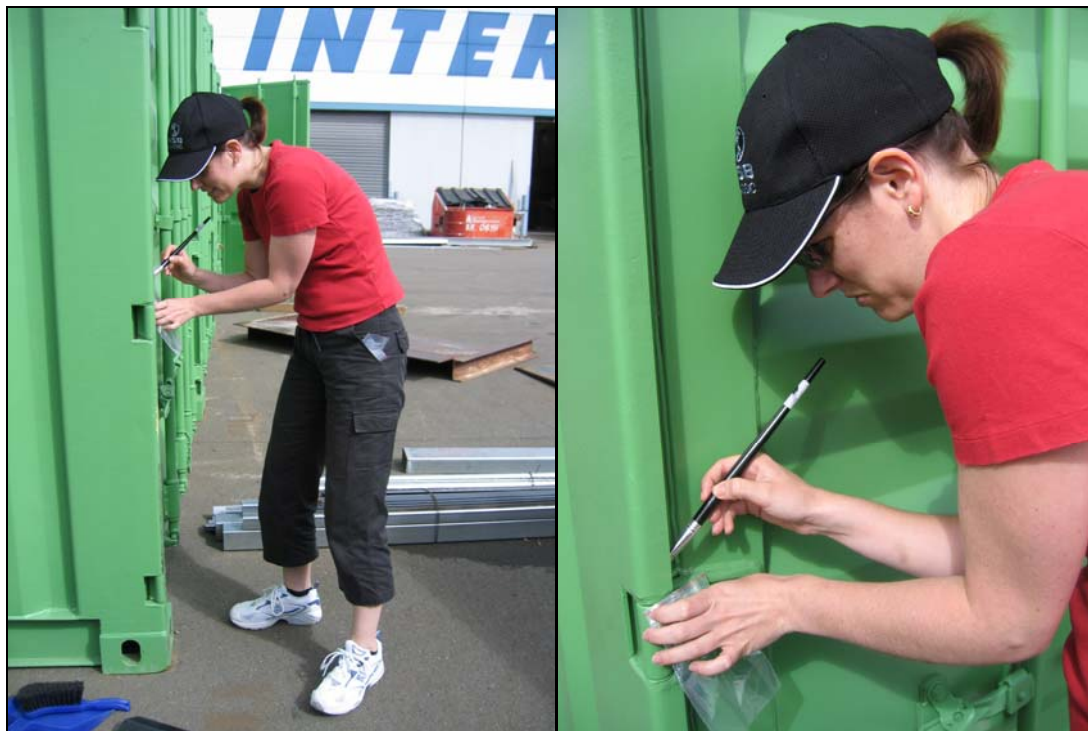
Figure 3.7 Manual inspection of the shipping containers at Antarctica New Zealand. Twelve containers were externally inspected using this technique (Photograph by A. Fortune).
