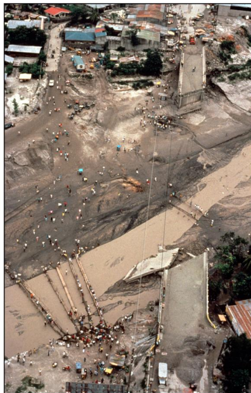
Figure 5: a) Only the roofs of 2-storey buildings are visible after repeated inundation by lahars following the 1991 eruption of Pinatubo, Philippines (C.Newhall).
