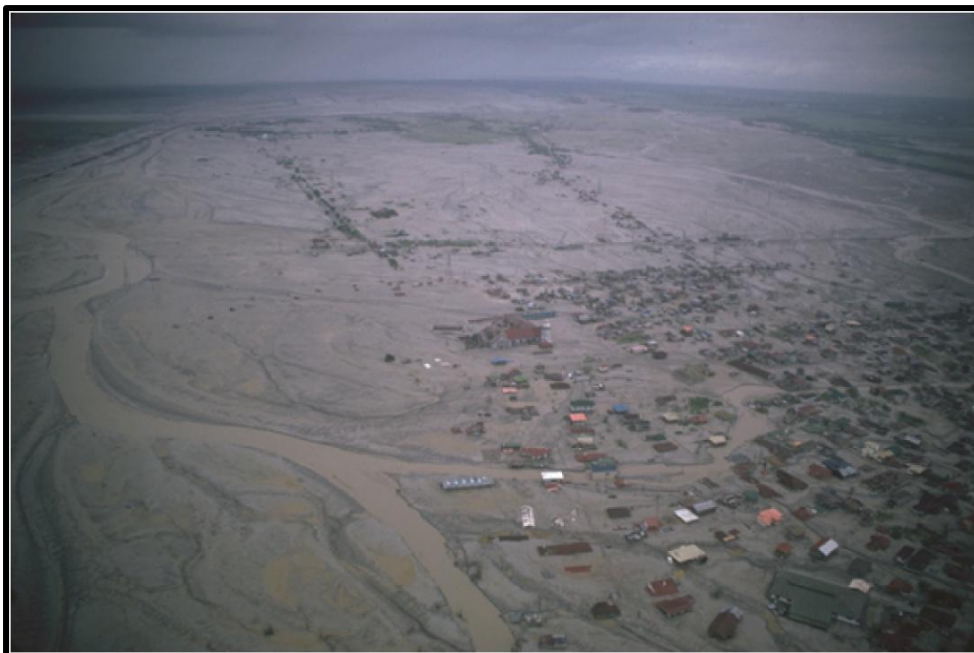
Figure 10 Lahars repeatedly buried the town of Bacolor from 1991-1995. Only roofs of 2-storey buildings are visible. Photo by Chris Newhall, USGS
