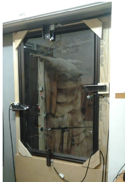
Figure 4.4 Transmission loss rig built for anechoic room doorway
