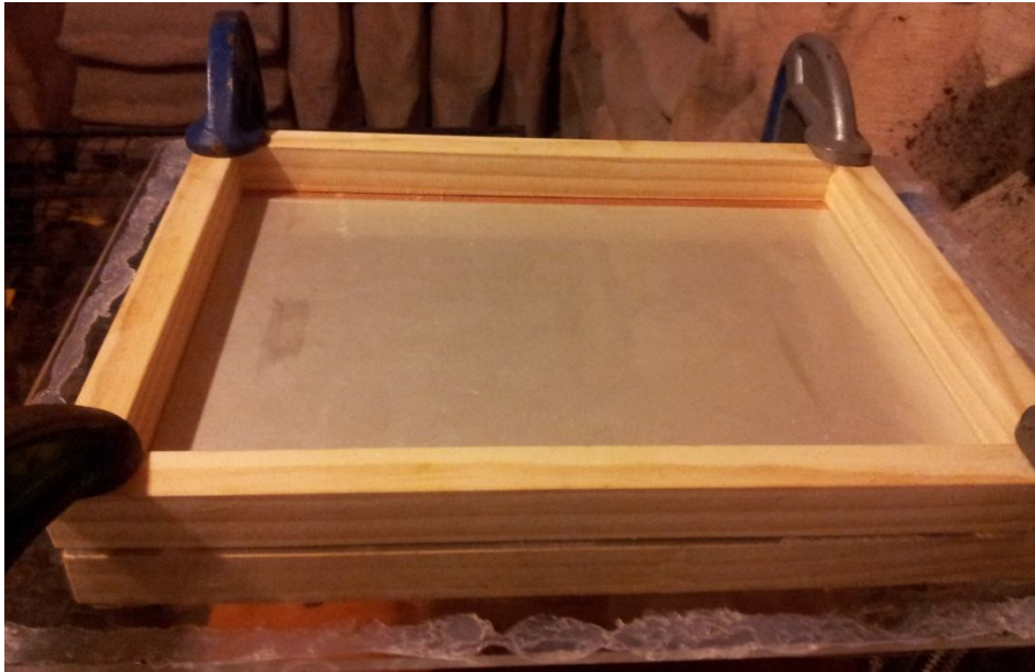
Figure 3.6 A completed window speaker using the vacuum construction method.
