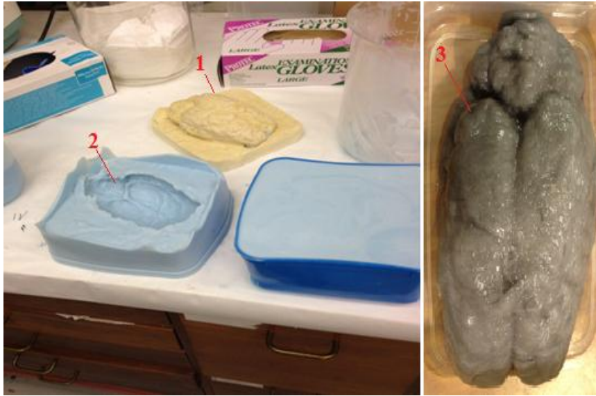
Figure 3-7: 1- dental stone model 2- Silicone mould 3- M1 in the shape of the bovine brain
