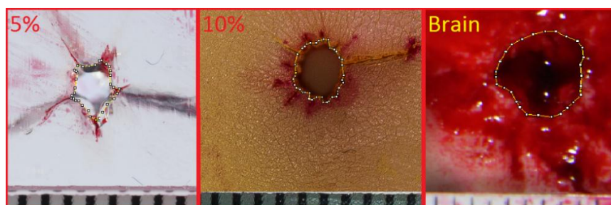
Figure 5-11: An example of polygon fit into the permanent cavity in different materials
