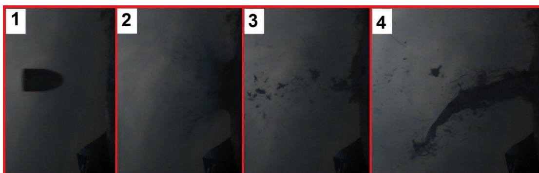
Figure 7-7: Sheep's head experiment: 1- Bullet before impact 2- Extrusion of the skin 3- Skin back to the original shape 4- Ejection of the brain
