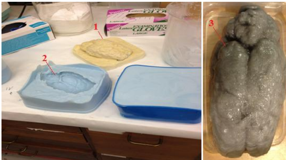
Figure 2-10: 1- Dental stone model 2- Silicone mould 3- M1 in the shape of the bovine brain
